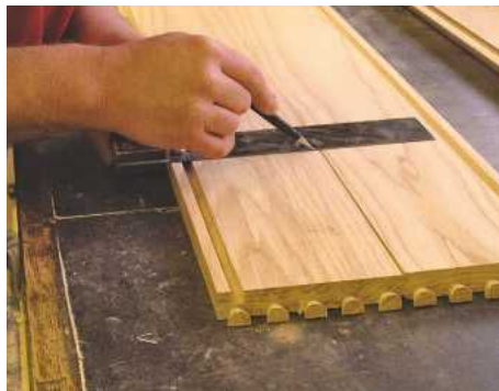
▲ Pic.13 Place the front uprights back-to-back and mark off the positions of the shelf sockets. Transfer these to the back upright
